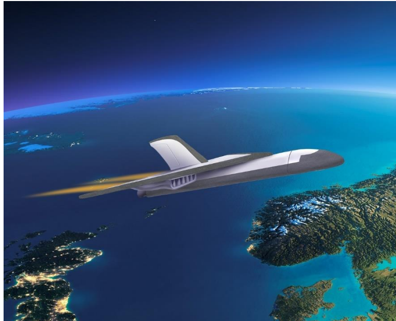
The Swala vehicle just prior to jettisoning its ramjets
